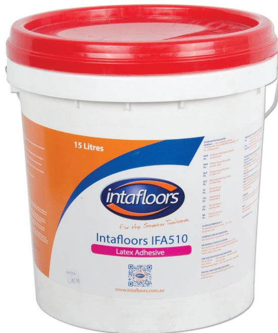
**INTAFLOORS IFA510 LATEX** is a compounded latex product used for the sealing of raw edges, strengthening worn backing, replacing damaged nap and adhering pad underlays to subfloors.
